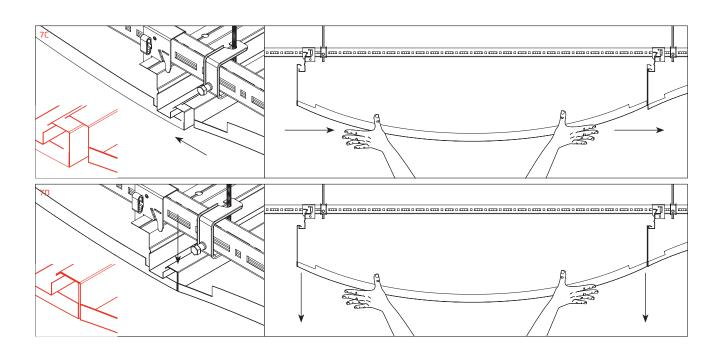
\*verify **interaxes** and **hanger models** according to the load at m² the antiseimic report and particular conditions when required. The **fastening** must be checked with regard to the loads, the anchoring base features and the installation accuracy, in order not to compromise the stability of the metal ceiling system. Lightings, accessories and systems must not weigh on the metal ceiling system, but must be independently suspended.
